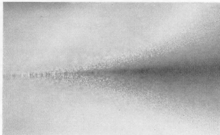
Figure 1. Filamentation of white offset ink with the Inkometer rollers turning at 300 feet per minute. The filaments reach a length of four-hundredths of an inch, forty times the thickness of the ink film. There is very little ink "mist."
