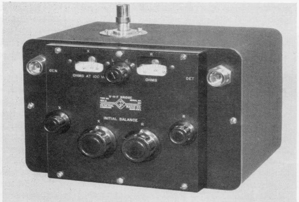
Figure 4. View of the engineering model of the V-H-F Bridge with coaxial adapter installed on the unknown terminal at the top of the cabinet. Panel size is approximately 11 x 9 inches. Production model has a larger ground plate around the unknown terminal and is equipped with carrying handles.
