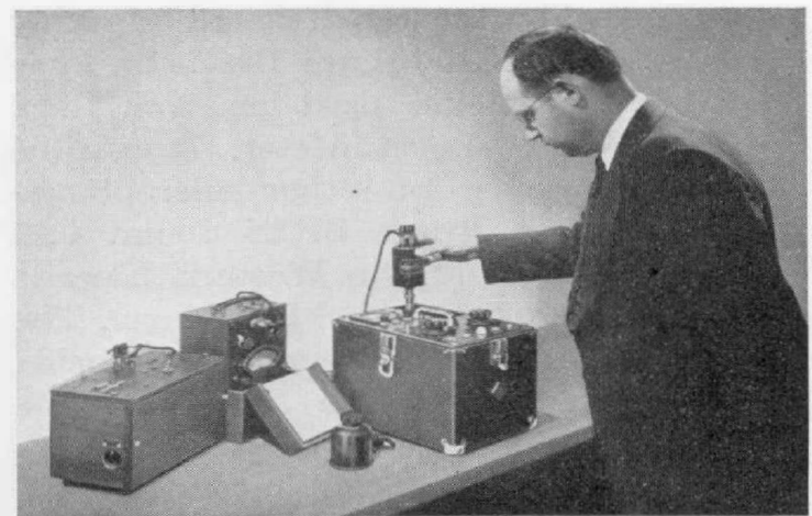
Figure 5. Calibrating a sound-level meter with the sound-level calibrator. A Type 723-B Oscillator and Type 727-A Vacuum-Tube Voltmeter provide the standard 400-cycle voltage.
