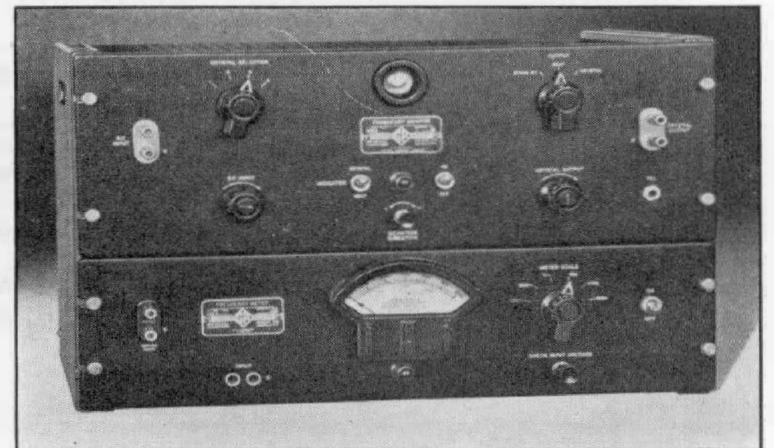
Figure 5. View of a Type 1175-B Frequency Monitor and a Type 1176-A Frequency Meter assembled in end frames.
