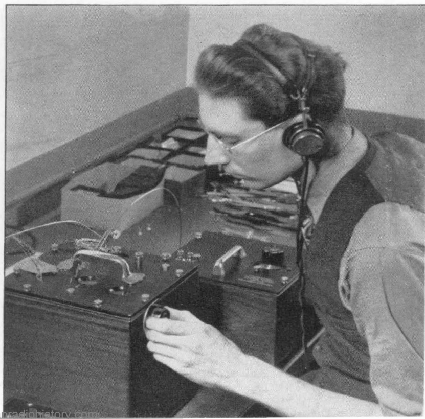
Figure 1. Calibrating precision capacitors in the General Radio Standardizing Laboratory.
