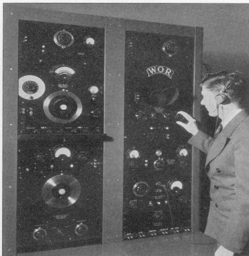
FIGURE 2. Equipment for measuring modulation and distortion consists of wave analyzer, beat-frequency oscillator, modulation meter, distortion and noise meter, range-extension filter, and cathode-ray oscillograph. These are conveniently mounted on a pair of relay racks as shown here.
