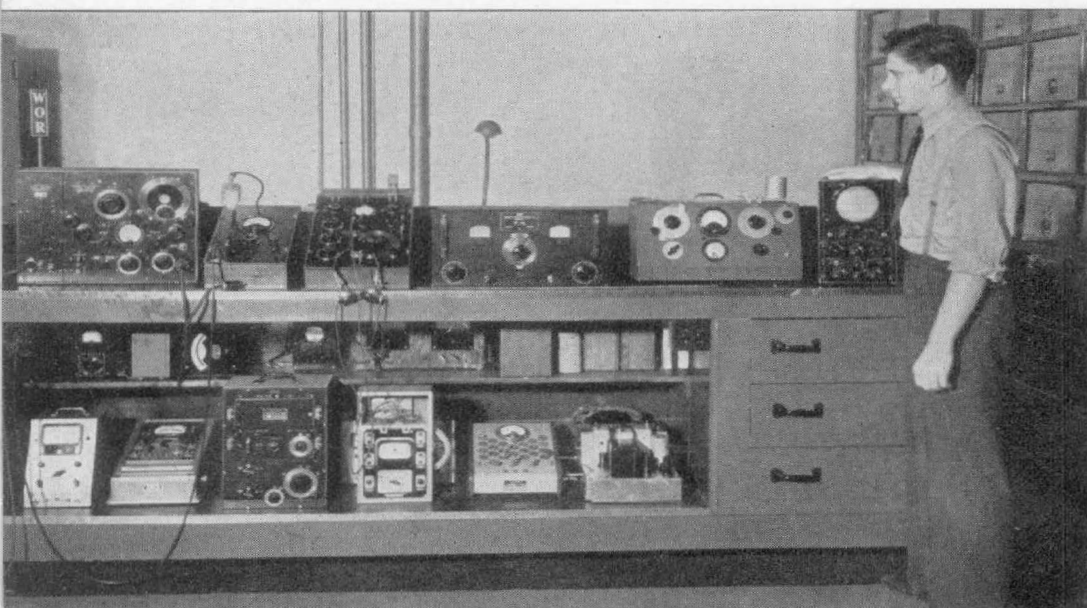
FIGURE 3. Equipment used on the test bench includes impedance bridges, vacuum-tube voltmeters, standard-signal generators, and other general-purpose test instruments.
