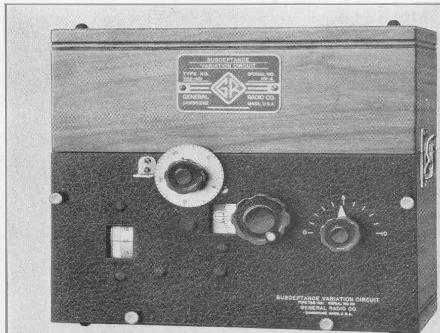
FIGURE 1. Panel view of the TYPE 755-AS1 Susceptance Variation Circuit.
