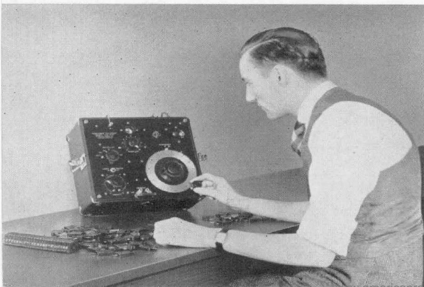
FIGURE 4. The capacitance test bridge set up for the rapid testing of mica condensers.
