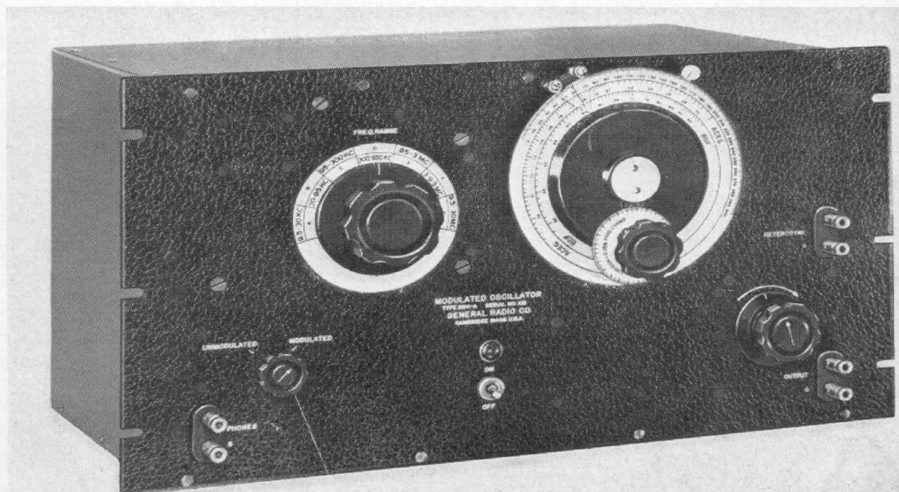
FIGURE 1. Panel view of the TYPE 684-A Modulated Oscillator
