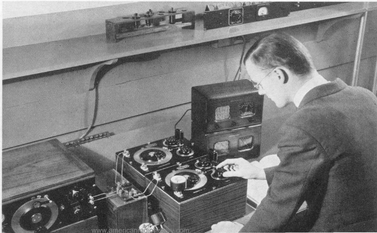
FIGURE 1. Two TYPE 721-A Coil Comparators arranged for testing coils at two frequencies.
