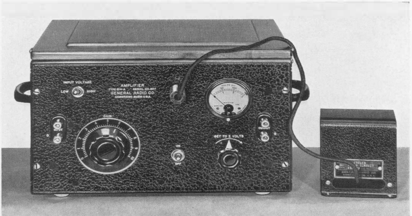
FIGURE 1. Showing how the tuned circuit is plugged into a jack on the amplifier panel
