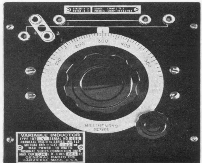
FIGURE 2. TYPE 107 Variable Inductor. Mutual inductance at any setting is one-half the difference of the scale reading and the value of self-inductance at zero mutual inductance as entered on the nameplate
