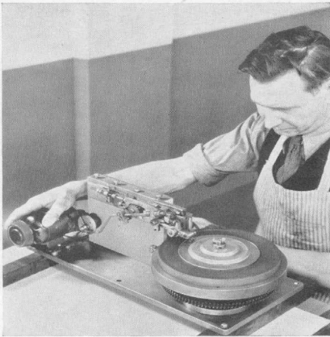
The self-indexing engraving machine which rules the scales on TYPE 704 and TYPE 706 Precision Dials
