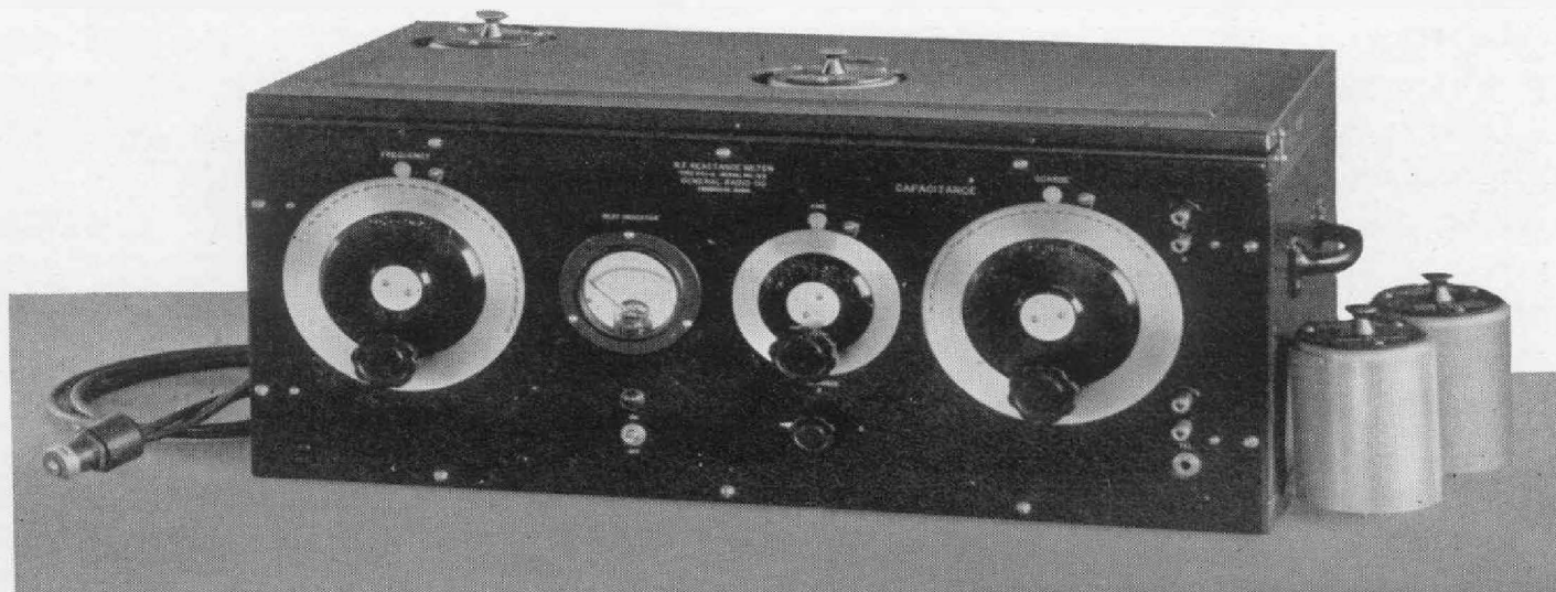
FIGURE 2. Front-of-panel view of the TYPE 421-A R. F. Reactance Meter. The dial at the left adjusts the frequency of the reference oscillator, the two at the right the "X" oscillator
