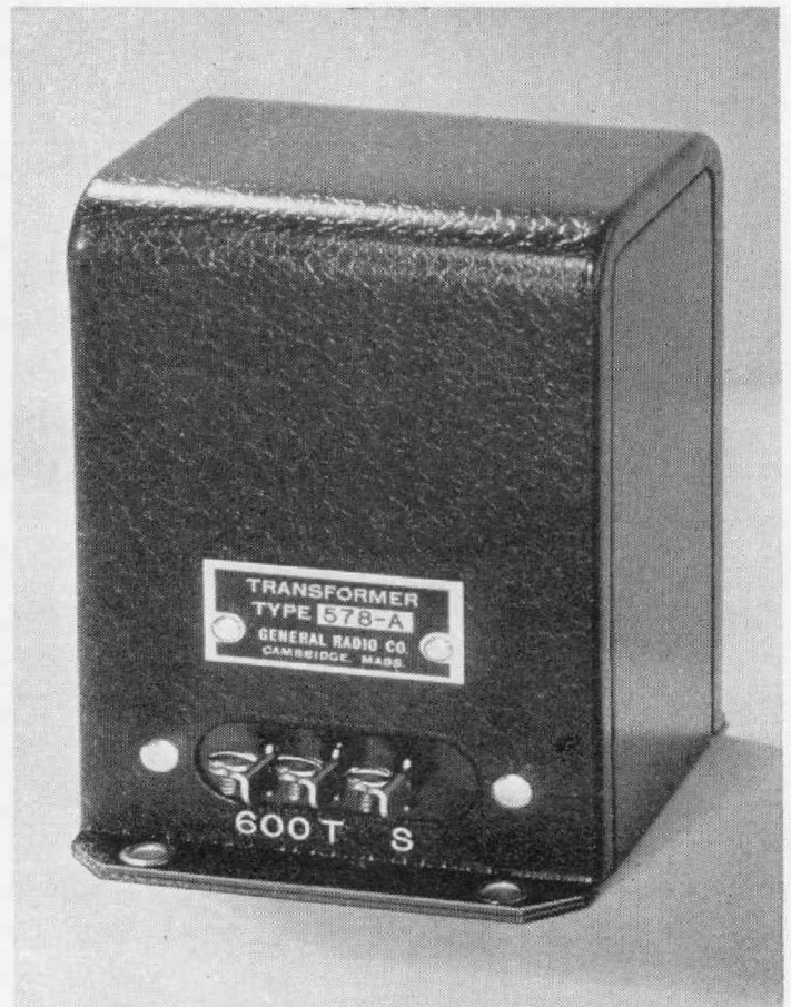
FIGURE 4. A mounted TYPE 578-A Bridge Transformer showing the terminal plate on the 600-turn side
