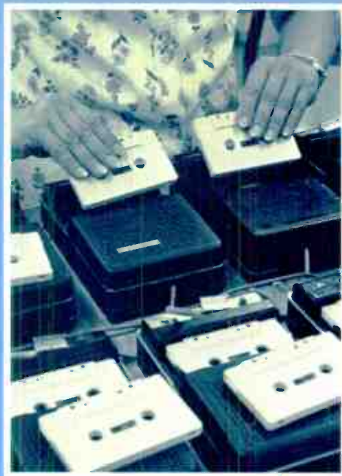
Quality control operator checks cassettes for mechanical functioning. At the next station, a sound check is made.
