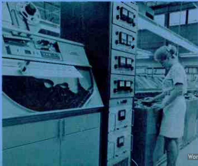
Ampex bin loop reproducer (BLM-200) drives ten cartridge slaves.
