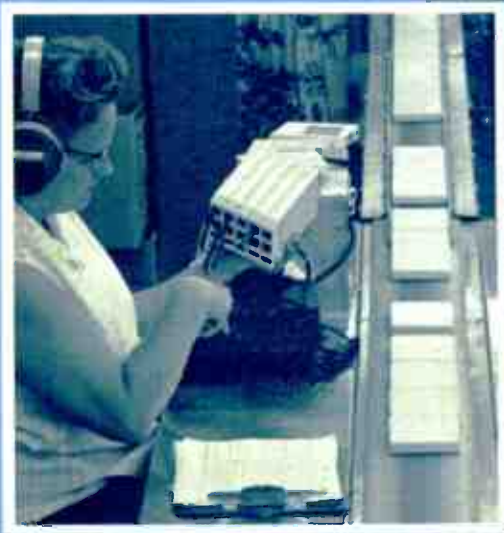
Following a stringent mechanical check, another quality control station makes a listening test.
