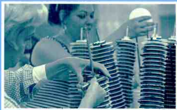
Album length reels are removed from the slaves for insertion into cartridges.
