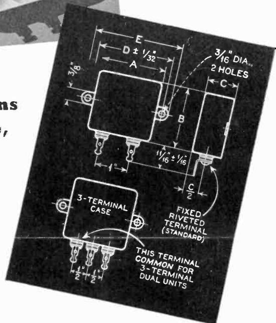
metal case with soldered bottom plate. Terminals are constructed with the Aerovox-originated "double-rubber" bakelite insulators permanently riveted to the case, making a sturdy, absolutely immersion-proof assembly. Terminals on side, top, bottom or ends to suit mounting and wiring requirements.
