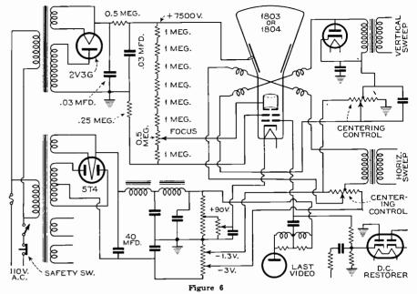
The high voltages employed in television receivers are dangerous. Precaution must be taken to prevent contact with the high potentials on the part of the "looker-in" as well as the serviceman. Even when the power is "off" danger exists, for, if the bleeder were open, the high-voltage condenser would retain its charge. The following measures are recommended:
