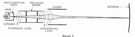
so-called "short" tube does not fulfill this requirement but the depth of focus is large enough to make the effect unnoticeable.
