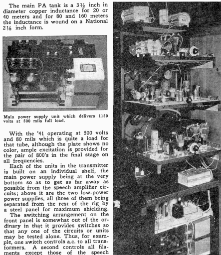
Rear view showing the three power supplies at the bottom and the modulator, exciter unit and final P A on the shelves above it.
