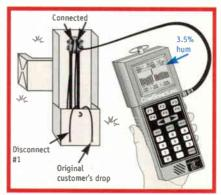
Figure 1: Unacceptable hum after disconnecting the first drop indicates one of the two drops still connected or feeder system is causing the problem
