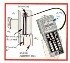
Figure 2: Hum modulation less than 2% after disconnecting second drop indicates that drop is causing the problem
