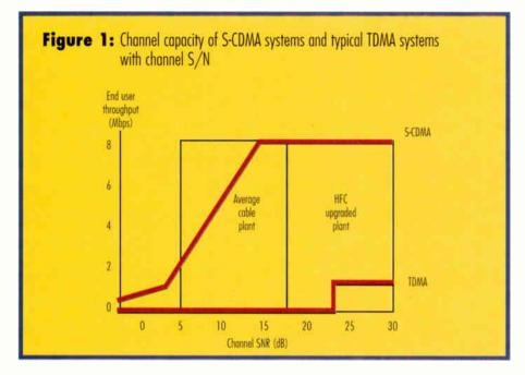
For any given set of noise conditions, an S-CDMA channel provides a more reliable upstream channel than a TDMA channel, which results in fewer interruptions in data transmission from excessive error rates. This higher channel reliability is a result of
