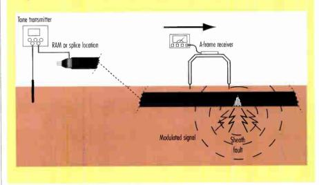
current flow from the fault to the transmitter, and when the operator physically steps over the fault, the current flow into ground at that location changes direction. (See Figure 4.) An indicator on the A-frame alerts the operator as to change in direction of the current flow. The location of the fault is now known and the appropriate actions are taken for sheath repair.
