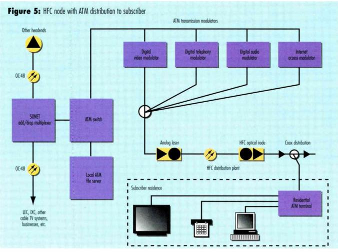
headend modulators, and from this point forward the distribution network looks just as it does today. The one exception shown here is the Internet access modulator, which transports ATM cells directly to subscribers' RF data modems.
