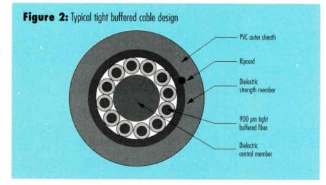
ments of the inside building environment. This makes tight-buffered cables susceptible to water penetration and migration damage when used outdoors. Bottom line, no plastic material is completely impervious to water, so a tight-buffer material alone cannot permanently isolate fibers from the influence of water. So, if water penetrates the cable jacket and subsequently freezes, individual fibers are subjected to microbending, increased attenuation or damage.
