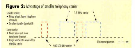
spare bandwidth required to do a carrier switchover in case of noise is also smaller. (See Figure 2.)
