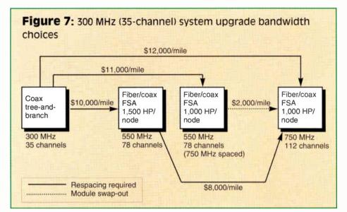
(bandwidth). Bob strongly recommends that you limit amplifier cascades to achieve a 49 dB C/N worse case (noise-free NTSC picture). Based on your average density of 80 homes/mile, this results in 1,500 HP/node at 550 MHz spacing and 1,000 HP/node at 750 MHz spacing. Although this is not where you project you will need to be some day (500 HP/node), you convince Bob that by allocating six fibers to each node, you can get there when you
