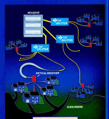
For CATV systems Gould has wavelength independent splitters with low insertion loss and high directivity (≤-65.0dB) -guaranteed for environmental stability and performance at the headend or in the field. Components are in stock in a variety of standard and customized package styles.
