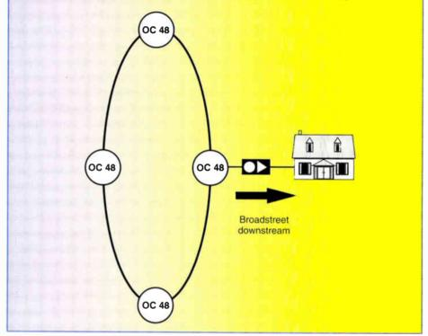
nect existing cable TV headends and gain seamless access to the public switched telephone network (PSTN). SONET is, in essence, a digital "superhighway," able to seamlessly pick up and drop off traffic at any node in the network. SONET's self-healing ring architectures are capable of protecting the traffic from a fiber break, equipment failure or catastrophic hub failure without any impact to telecommunication services.
