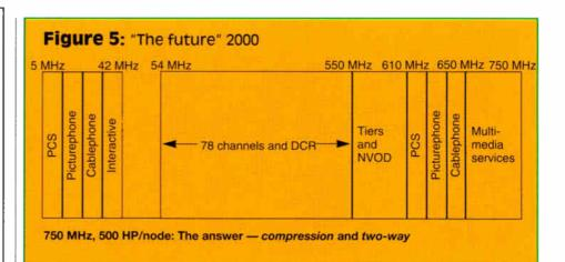
digital terminal has been authorized to decode the signal. This concept of segmenting the system such that viewers in different serving areas can each watch a different program using the same spectrum allocation is identical to the method used in cellular phone systems. It is called frequency reuse. Your boss is a quick study and he then asks the \$64,000 question: How much bandwidth is enough and how deep in the system do you have to take fiber?
