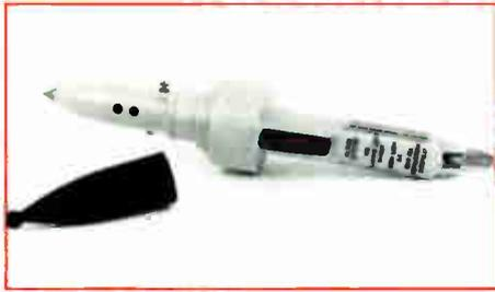
use in the testing of various conductive objects that might expose craftspeople to electric shock. It is battery-powered, self-contained and may be hung from a work belt when not in use.
