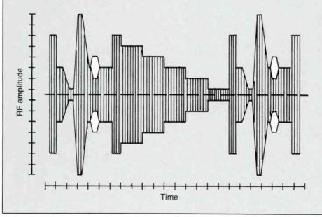
amplitude of 100 IRE. The 100 IRE signal pulse remains at 100 IRE for about  $2 \,\mu s$  before returning to 0 IRE.
