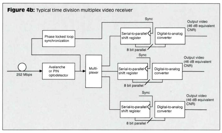
a single transmitter output; a regular time slot is assigned to each PCM channel. The PCM channels can then be grouped together into a time sequential format (serial). A complete sequence that samples each of the input analog channels is called a *frame*.
