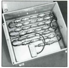
Typical multitrap assembly. The subscriberpowered amplifier counters cumulative trap loss.
