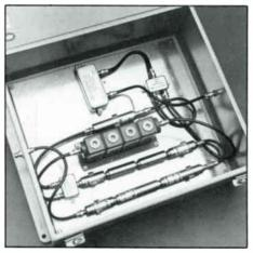
This multichannel trap assembly uses a special bandpass filter to isolate a desired super-band channel.
