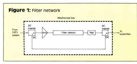
and capable of being mounted on the house or on the pole. This is usually the highest cost component of such a network, since many channel cherry-picking menus can be managed with correct selection of pay TV and tiering filters. The accompanying photos reveal typical housed networks.
