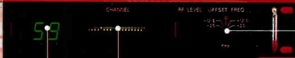
Large green LEDs display accurate channel indication.
