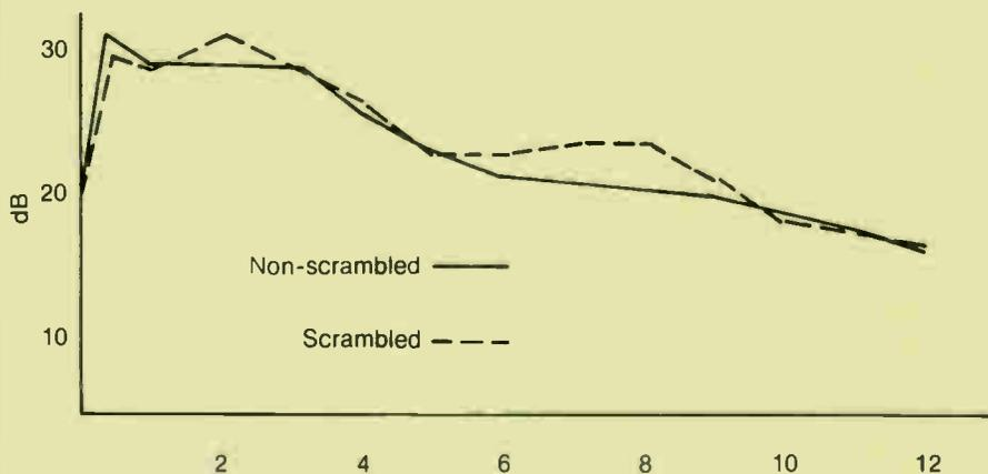
**Figure 7:** Comparison of sine wave sync suppression, scrambled vs. non-scrambled (consumer decoder)
