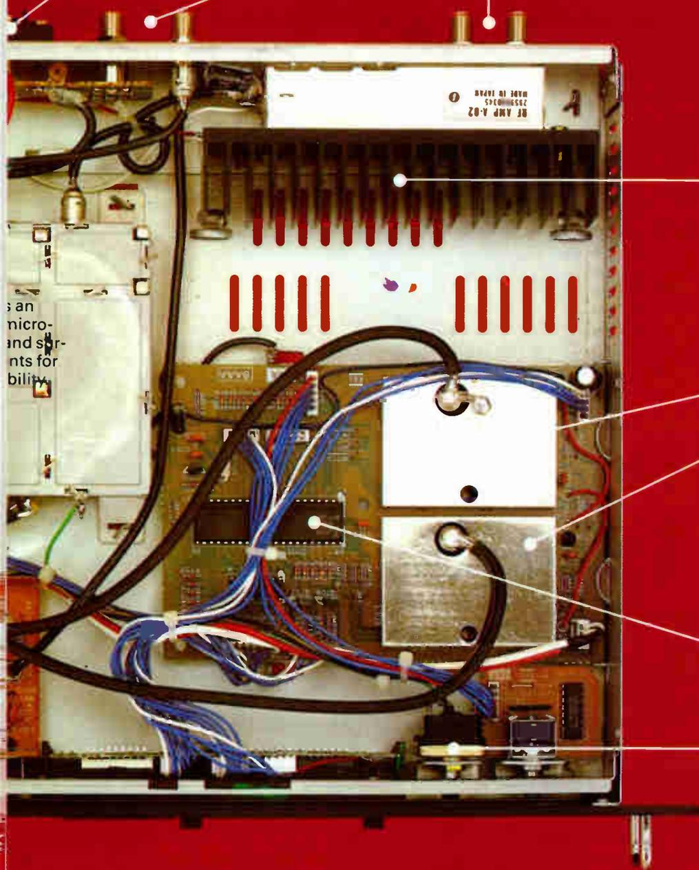
Low noise, hybrid power, push-pull amplifier that is adequately heatsinked and fully shielded.
