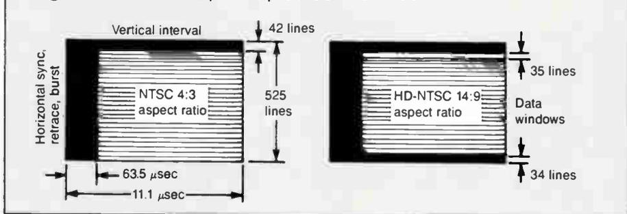
**Figure 4b: 14:9 aspect ratio viewed on an NTSC receiver**
