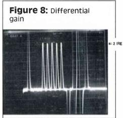
largest chroma envelope (spike) is 100 IRE. Measure the difference between the peak step and the smallest step. This is the differential gain. The parameter is not to exceed 15 IRE.
