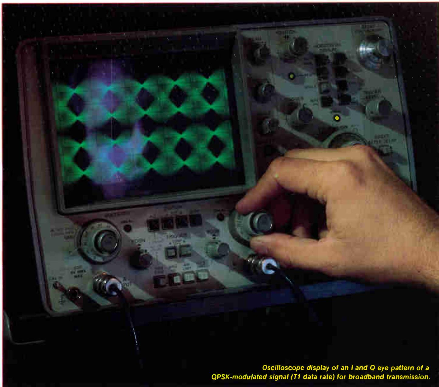
Oscilloscope display of an I and Q eye pattern of a QPSK-modulated signal (T1 data rate) for broadband transmission.
