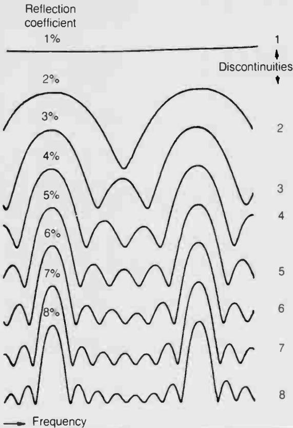
**Figure 83:** Reflection vs. frequency—three reels of CATV cable showing effects of periodicity
