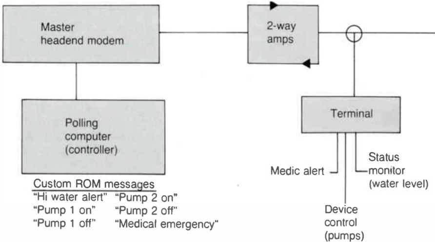
'The equipment required to make a system interactive is uncomplicated and inexpensive, assuming the cable plant has two-way capability'
