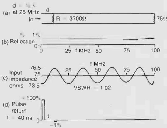
**Figure 79:** Uniform lossless line, terminated, two discontinuities
