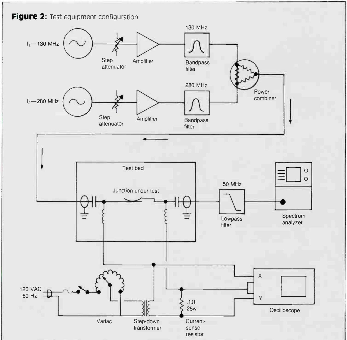
were searched for. None were found down to the noise floor of  $-80$  dBm. This performance is adequate for the testing described in this article.
