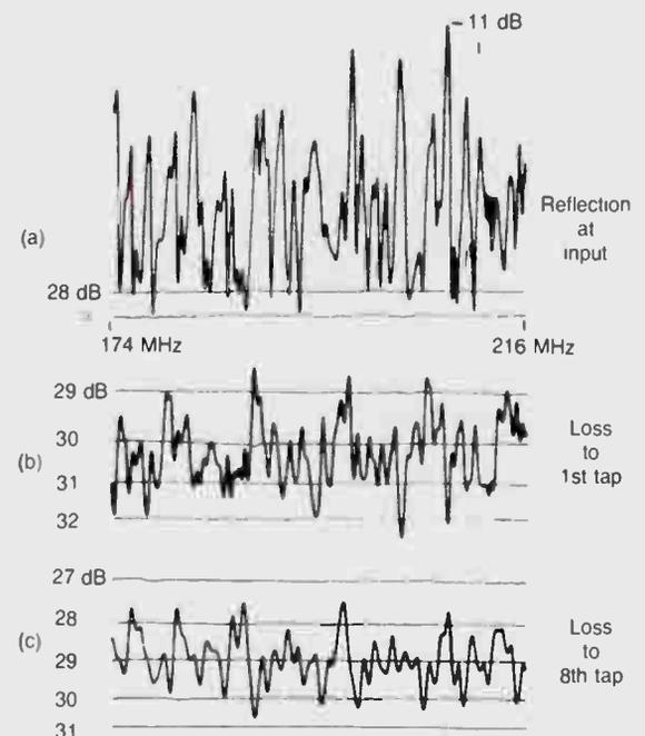
**Figure 88:** Reflection vs. frequency—BMT pressure taps on 1/2-inch cable
