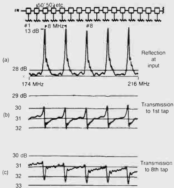
**Figure 86:** 16 BMT taps on 1/2-inch feeder 800 feet long, hi-band performance (there was one tap in each 50-foot cable section but spacing was random)
