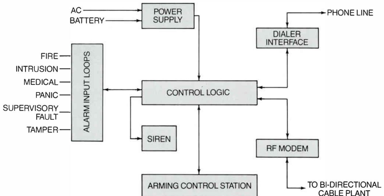
technology has evolved. Today, it is possible for home alarm terminals to monitor multiple zones for intrusion, smoke and heat or panic alarms (fire, medical or assault). Distinct condition-type alarms also can be transmitted to indicate signal loss, low battery and tamper.
