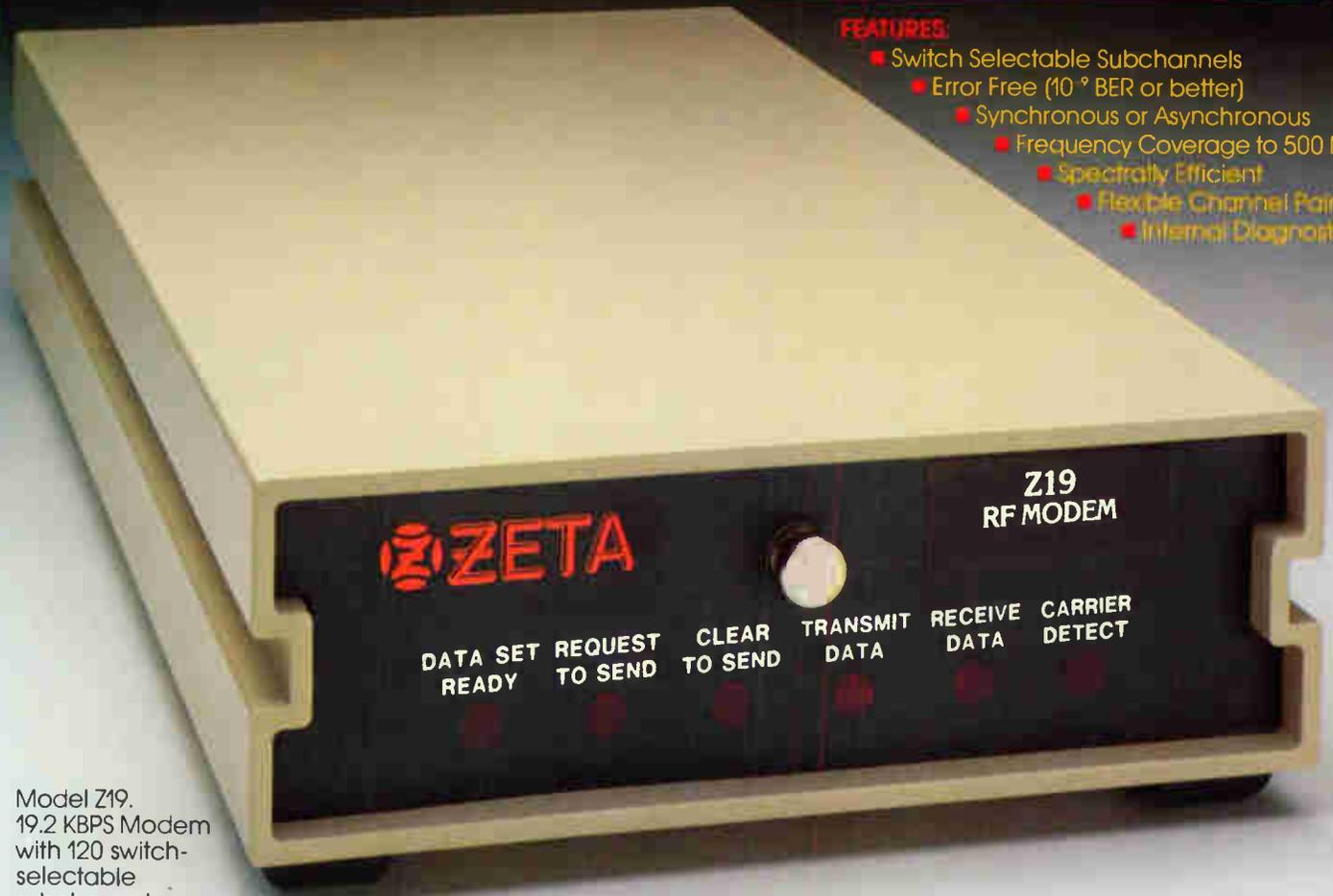
Model Z19. 19.2 KBPS Modem with 120 switch-selectable subchannels.
