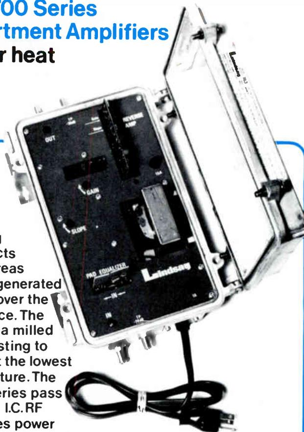
The heavy wall aluminum casting efficiently conducts heat away from areas where it is being generated and dissipates it over the entire outer surface. The I.C. is attached to a milled surface of the casting to keep the flange at the lowest possible temperature. The combination of series pass power supply and I.C. RF circuitry minimises power consumption and decreases heat generation.
