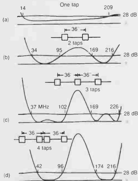
**Figure 89:** Reflection vs. frequency—four pressure taps in various possible arrangements
