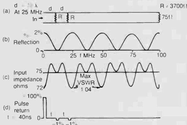
**Figure 80:** Uniform line, terminated, two equally spaced discontinuities; 4 equally spaced discontinuities
