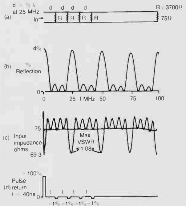
**Figure 81:** Uniform terminated line, eight equally spaced discontinuities
