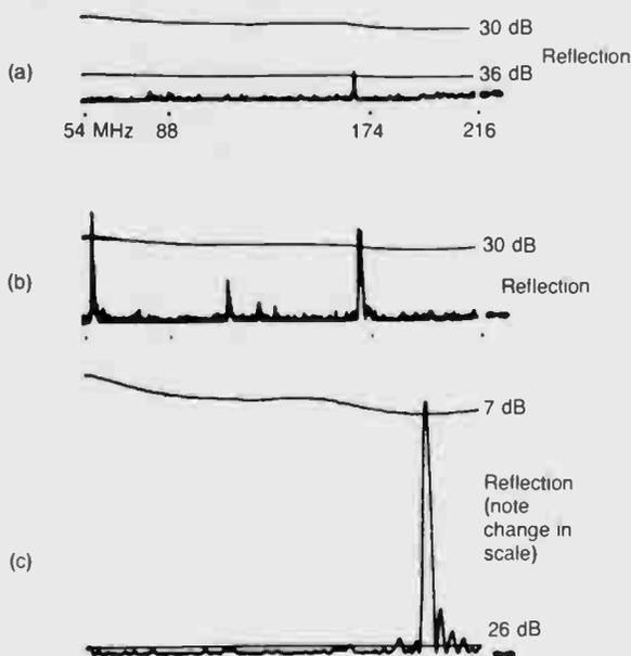
**Figure 84:** Addition of reflections, pressure taps spaced at 50-foot intervals along 1/2-inch foam cable
