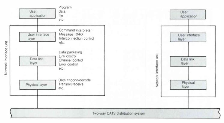
cast" downstream data, identifying data packets addressed to it, transferring the associated data to the user device. A block diagram of the NIU is shown in Figure 4.
