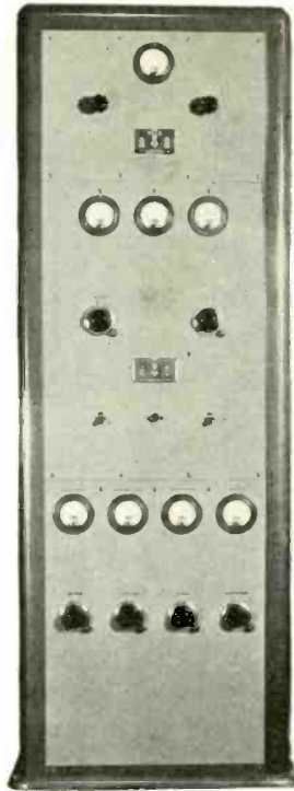
FIG. 7. FRONT VIEW OF THE 250-E TRANSMITTER. THE PANEL AT THE TOP CONTAINS THE HIGH-LEVEL MODULATION UNIT.
