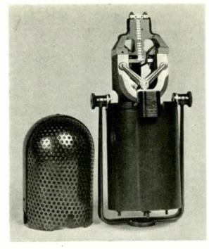
FIG. 3. THE UNI-DIRECTIONAL MICROPHONE WITH OUTER Shield Removed.
