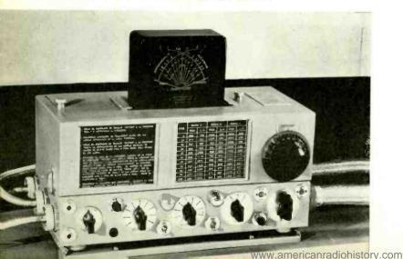
to provide for the pilot automatic and continuous information on his position in space with respect to the airport. This information must be three-fold: in what direction the airport lies; how far down; and how far away.
