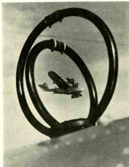
A CLOSE-UP VIEW OF THE DIRECTION FINDER LOOP ANTENNA ON A DOUGLAS AMPHIBIAN.
