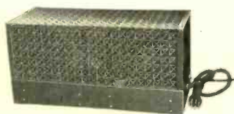
2A3 power supply with perforated protective cover fully mounted.
