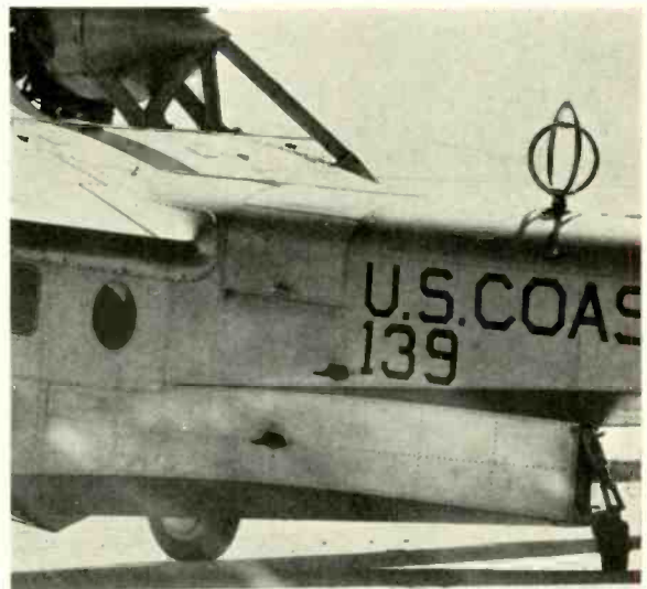
COAST GUARD PLANE — EMPHASIZING THE DIRECTION FINDER LOOP ANTENNA.
