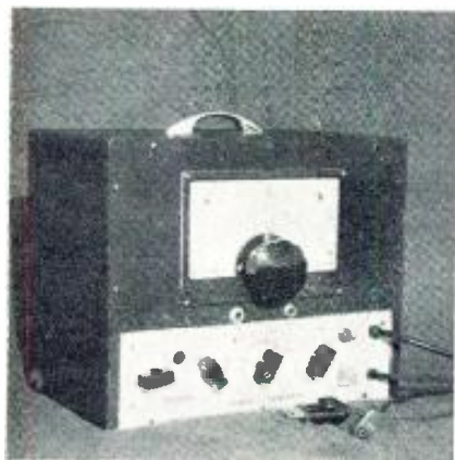
Front view of signal generator. Controls are, from left to right: Zero set variable capacitor, bandswitch with four positions, modulation with 30%, 50% and 100% points marked, r-f output 1000-ohm control with the power switch on the same shaft, and a lo-hi output toggle switch which can be seen above the small scale neon on indicating light.
