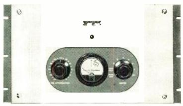
**Type 89.4.** Chassis construction is for vertical rack mounting. Removable front panel for easy access to all circuits. Meter and selector switch provide convenient indication of output level at 1000 cps and current readings of all tubes.
