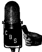
Left: Microphone with "P-42" Receptacle and P-CG-11 Plug used for platform public address. (Photo courtesy Reiss P. A. Systems, Detroit). Right: Mike used by CBS-Hollywood, with P-CG-12 plug shown in hand. As in the case of the above Type "O", two mating "P" plugs can be used conveniently for cable extension where receptacle is not an integral part of the microphone itself.
