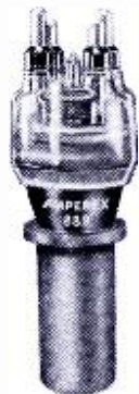
Amperex Type 889-R Transmitting Tube. Filament voltage, 11 volts. Filament current, 125 amperes. Amplification factor, 21. Direct interelectrode capacitance: grid to plate, 20.7 \mu\text{f} ; grid to filament, 19.5 \mu\text{f} ; plate to filament, 2.5 \mu\text{f} . List price, $325.00.
