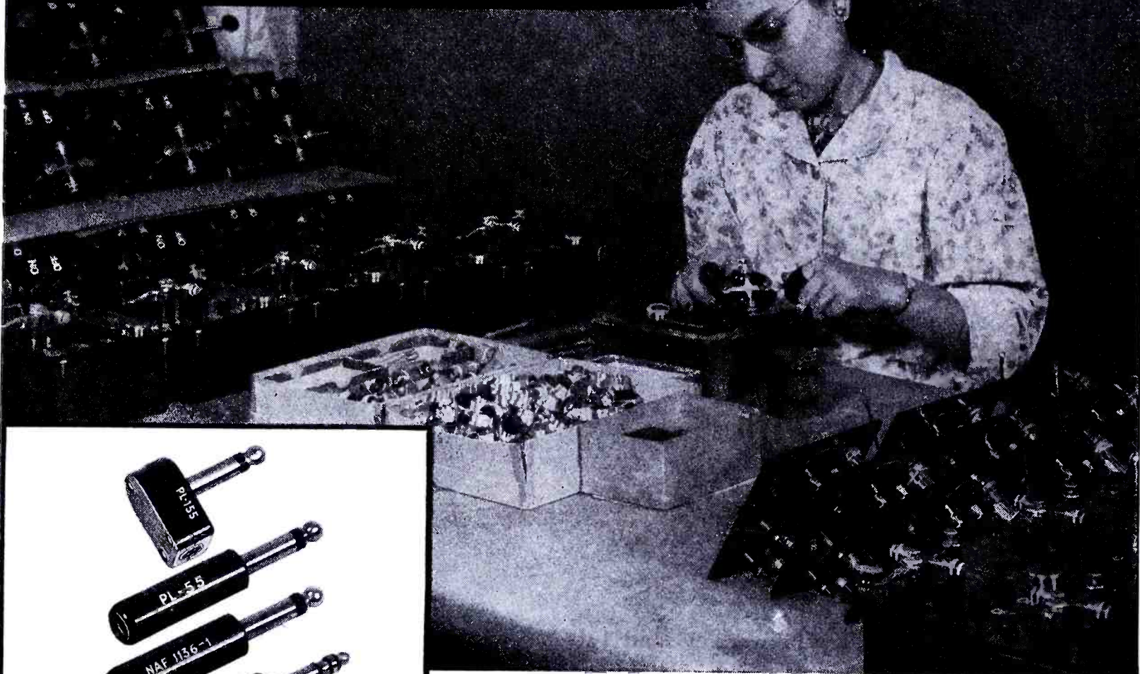
Final operation in assembly of a 110-volt radio control unit. Metal and plastic parts made by Remler.
