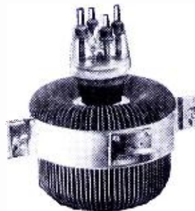
Amperex Type 889-R Transmitting Tube. Filament voltage, 11 volts. Filament current, 125 amperes. Amplification factor, 21. Direct interelectrode capacitance: grid to plate, 20.7 \mu\text{f} ; grid to filament, 19.5 \mu\text{f} ; plate to filament, 2.5 \mu\text{f} . List price, $325.00.
