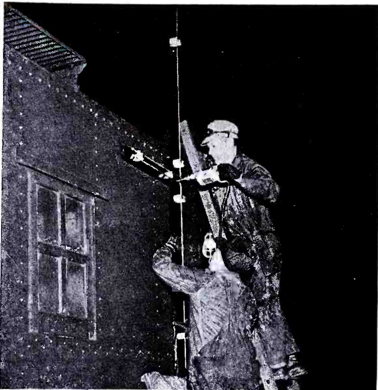
Figure 1 Installing the two one-half-wave in-phase antenna array on the caboose of a Denver and Rio Grande Western freight train.
