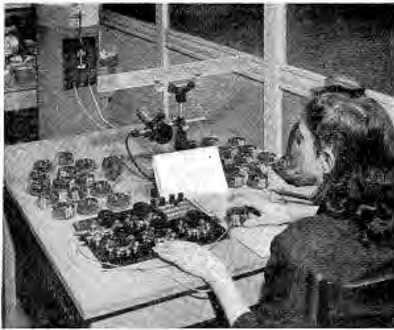
Left, attenuator windings receiving a galvanometer test. (Courtesy Daven) Right, a Clarostat type attenuator.
