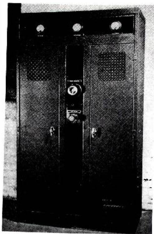
Figure 5 The completed power supply in case designed to match the transmitting equipment.
