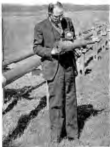
Figure 2 Dr. Southworth with one of the resonant chambers used for tests for wave guide transmission. Behind him are two experimental wave guide transmission lines.
