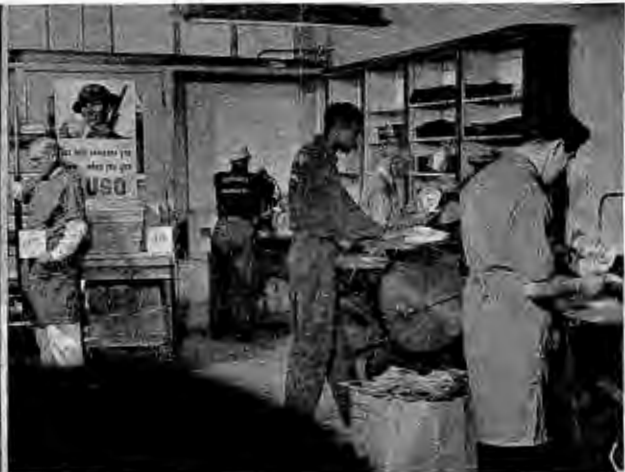
Making of the paper disc records, on which photographed and written messages are printed. At left, we see the drying room, while at right, the cutting operation is shown
