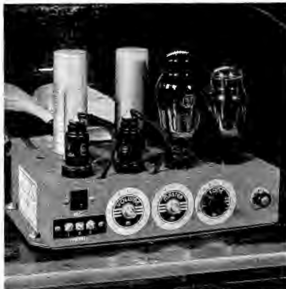
A closeup of the line amplifier, having 15 watts of power. It feeds the leased telephone line through a 500-ohm matching transformer at approximately zero level.
