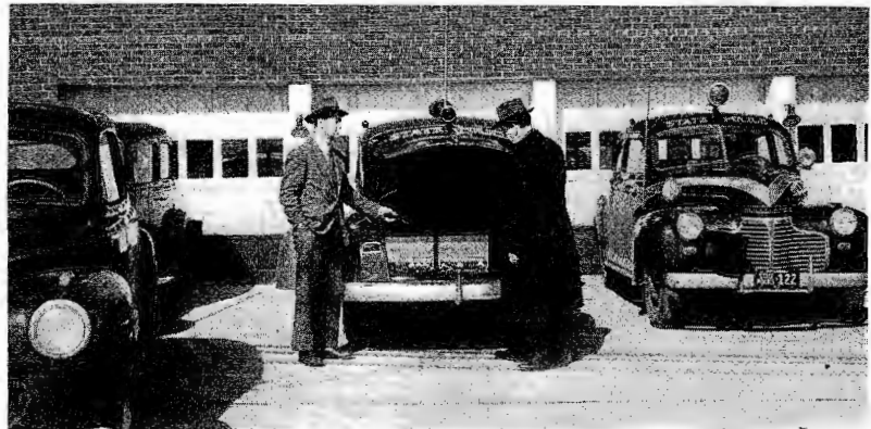
260 PATROL CARS USING 50 WATT TRANSMITTERS AND 2 CRYSTALS FOR DUAL-CHANNEL 3-WAY OPERATION
