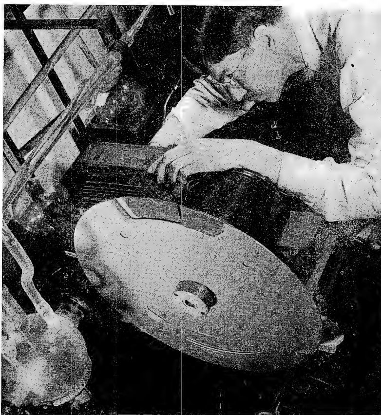
Lightning arrestors seem to be simple devices. Yet their design and operation is involved; so much so, that Westinghouse engineers developed the arrangement shown above to make a photographic record of an electric arc in 1/10,000 of a second of its flight.
