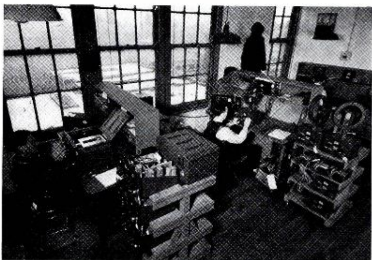
Fig. 8. The final step is test laboratory where each receiver is instrument and on-the-air tested.
