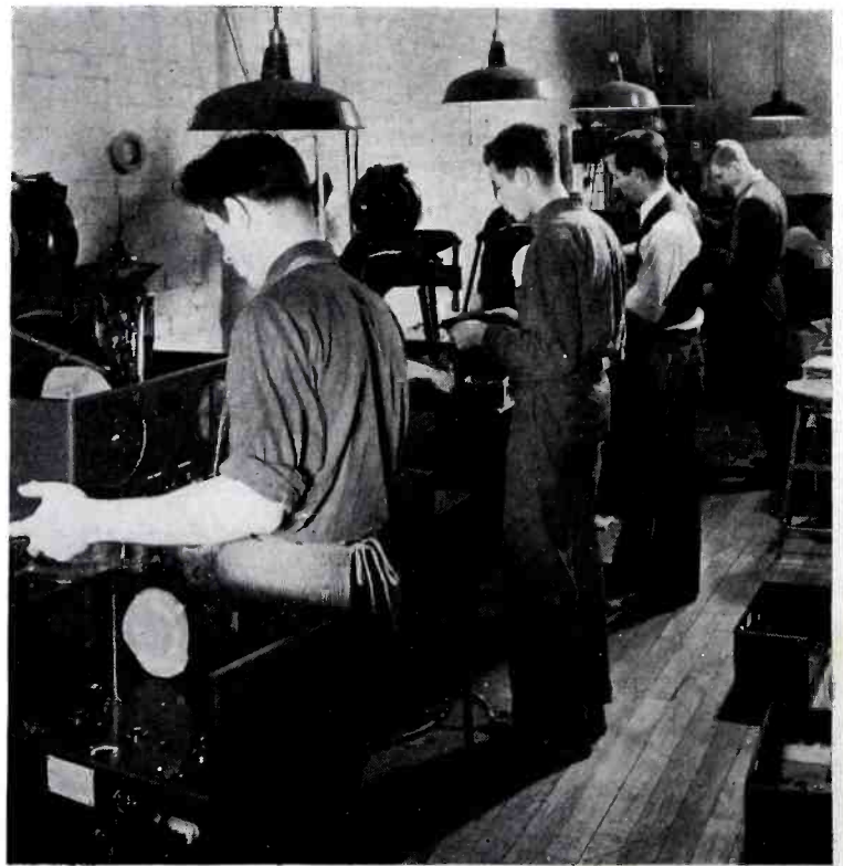
Fig. 3. Riveting machines make quick work of mounting sockets, terminal strips and the like.
