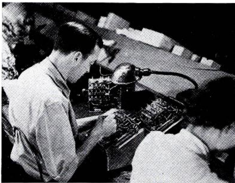
Fig. 6. At short distances along the production line an inspector checks work of operators immediately preceding.
