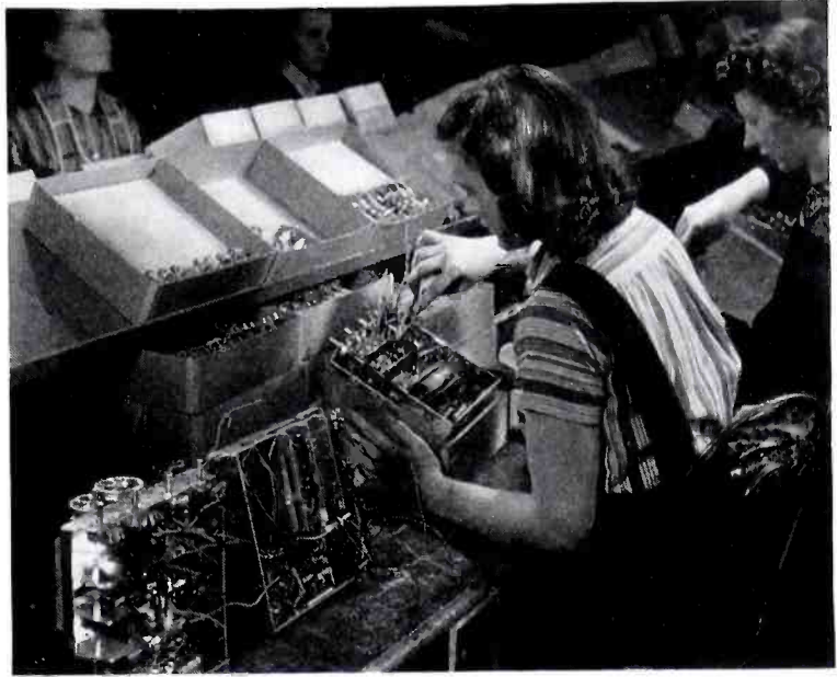
Fig. 5. This girl mounts 3 r-f coil assemblies. Operators following will wire these.
