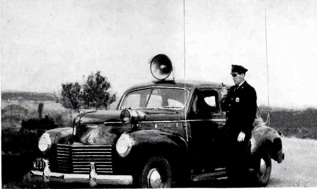
Fig. 6. A view of the car showing the separate transmitting and receiving antennas.
