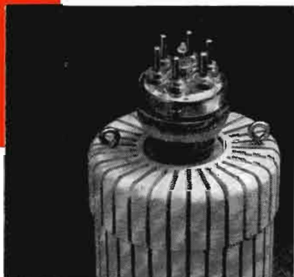
The tiny GL-8002-R used in the 3000-watt FM transmitter was specially designed by G-E engineers for ultra-high-frequency application. It has a center-tapped filament and three grid-leads. Output: 1800 watts up to 120 mc.
