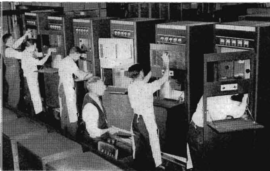
One-kilowatt frequency-modulation transmitters in various stages of completion at G-E Schenectady works.
