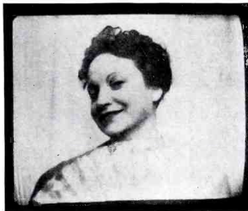
Fig. 22. Photo of French television image, 450 lines interlaced, 50 fields.
