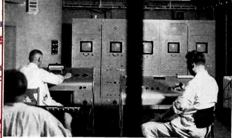
Fig. 34. (Above) Studio sound and vision control desks (Telefunken).
