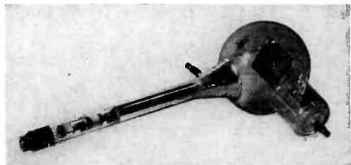
Fig. 14. (Below) A 40-kv Safar tube for projection receivers.
