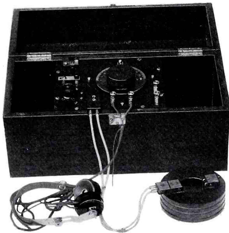
An early type of wavemeter. Compare with modern instrument at left.
