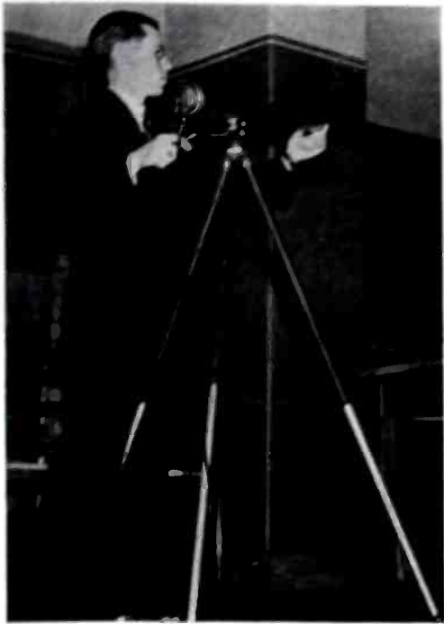
R. N. Marshall, of the Bell Telephone Laboratories, demonstrating a unidirectional microphone.
