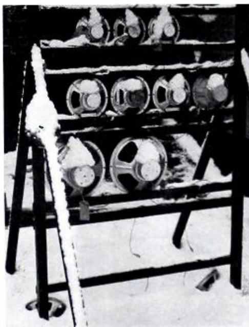
These speakers are being tested for their rust- and dust-proof qualities.
