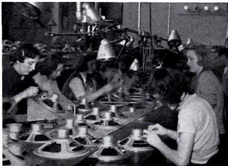
Lower left: Approaching the end of the assembly line. Lower right: Another part of the speaker assembly line.
