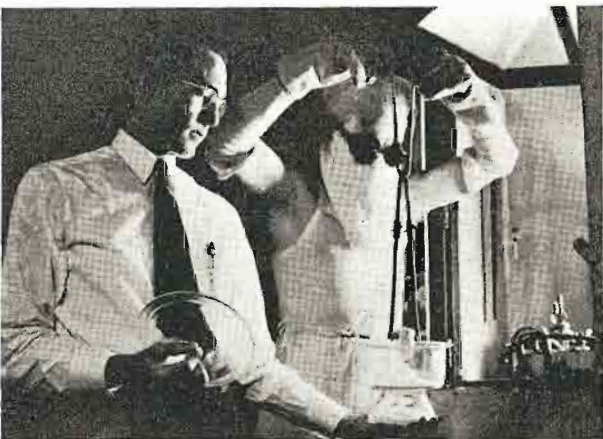
Below: Fig. 8. Removing fluorescent material from a furnace. RCA photo.
