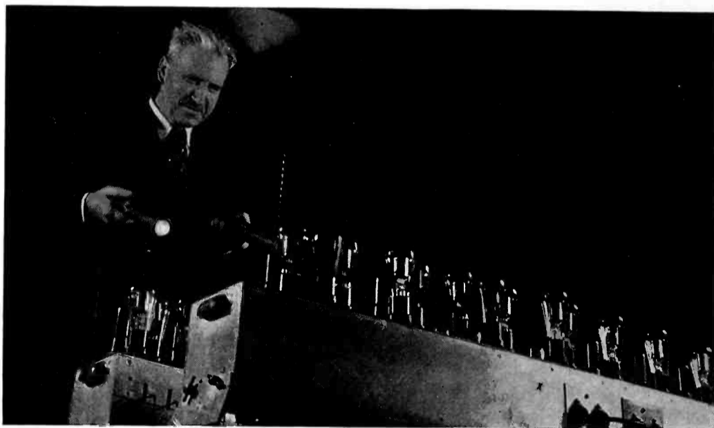
Playing marimba with light beams at Westinghouse exhibit. Hammers are operated by relays energized by photocells.
