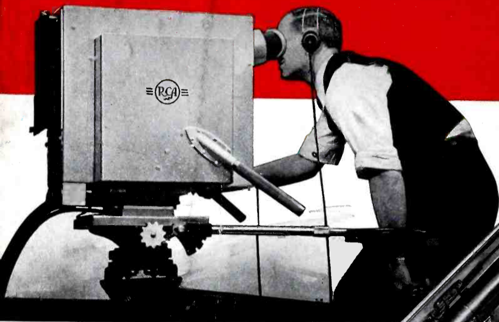
Television transmission with the RCA 1850 Iconoscope under studio conditions. A lens in the "camera" focuses the scene on the photosensitive mosaic of the "Ike".
