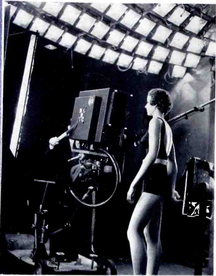
The lens, lamp and reflector array as seen from the television stage.
