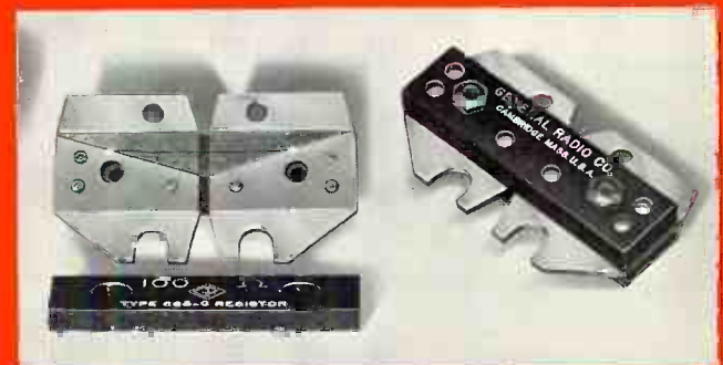
In the Type 663 Resistors the wire is clamped on flat metal fins to decrease inductance and increase power dissipation
