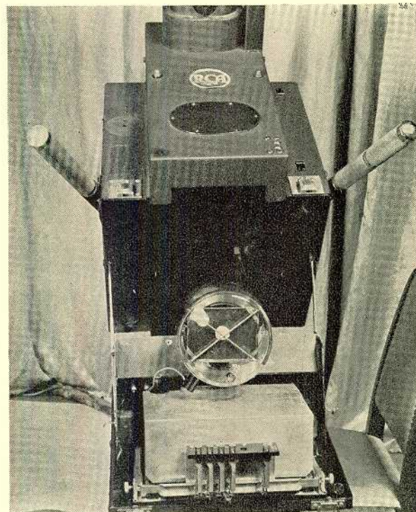
Another view of an open television camera. Note that iconoscope shield has been removed. NBC photo.
